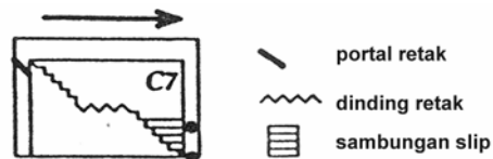
C Diagonal crack
